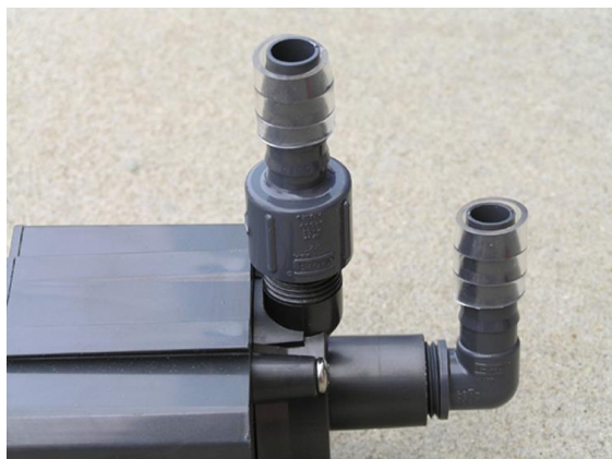
Figure 11. Clear flexible tubing will ensure a snug fit for tubing going to the biofilter
