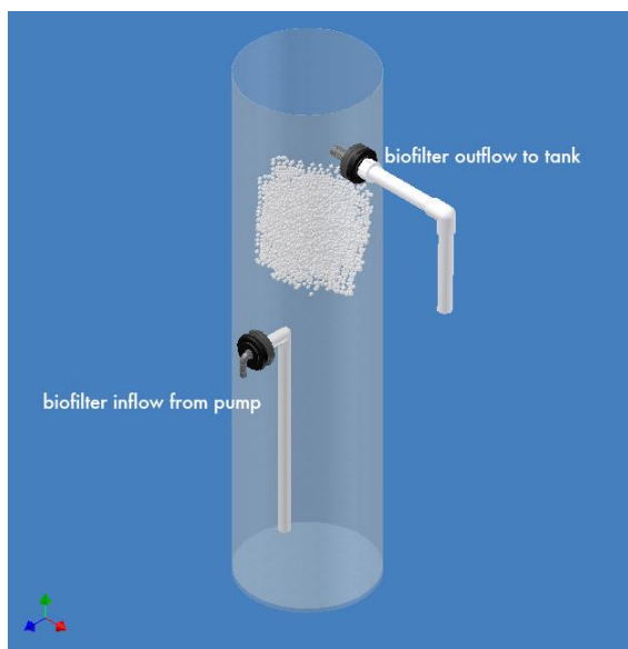
Schematic 3. Compare your biofilter installation to this diagram
