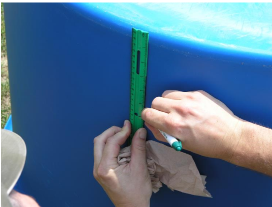
Figure 3. Cut a hole for the 2" bulkhead
