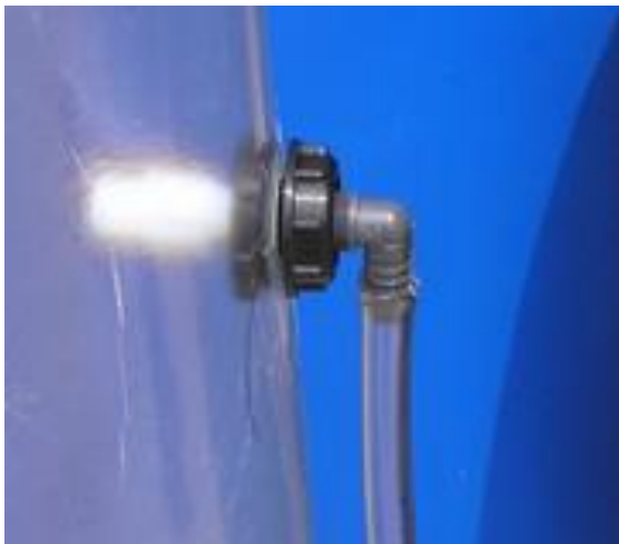
Figure 14. Rotate the male 90° ell so that it points straight down
