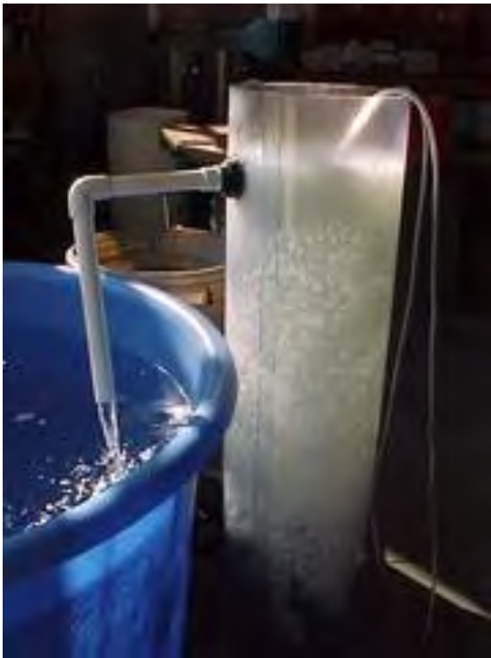
Figure 25. Orient the biofilter so the outflow pipes are going into the tank
