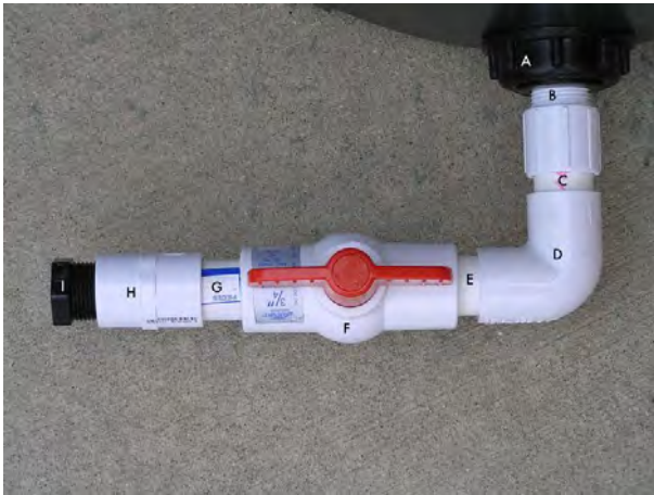
Figure 8. Adding a 3/4" male plug (I) to seal off the drain is optional but can be added insurance against leaks or accidentally leaving the ball valve open
