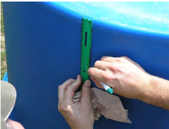
Figure 3. Cut a hole for the 2" bulkhead
