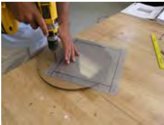
Figure 20. Drilling at a steady speed will help prevent cracking
