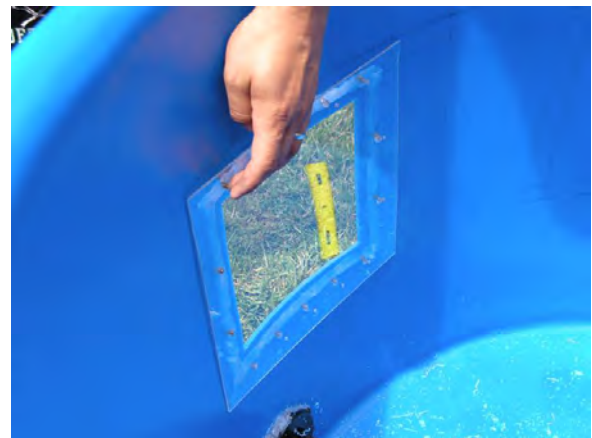
Figure 22. Apply silicone and attach with nuts and bolts
