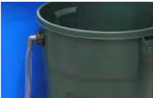
Figure 9. When installing the external plumbing, be sure the 90° ell and the tube are perpendicular to the floor
