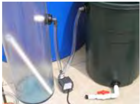
Figure 24. All tubing should be as straight and as free from kinks as possible to allow unobstructed flow
