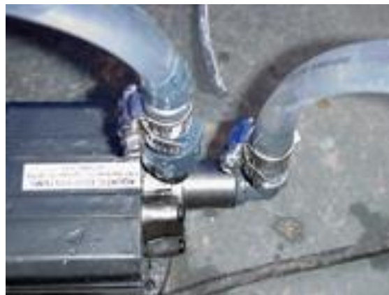
Figure 12. Use hose clamps to secure clear flexible tubing
