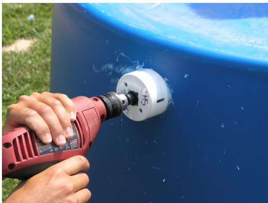
Figure 3. Cut a hole for the 2" bulkhead
