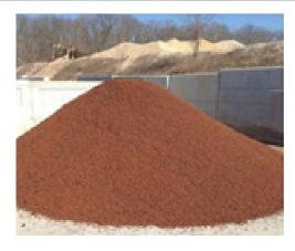
media contained 98% less carbon than traditional heatexpanded media. Platformscale analysis quantified the stormwater retention capacity of the brick-based media. About half of the storm events monitored created runoff. For events that did result in runoff, brick-based media retained at least 60% of the event, with the exception of Hurricane Sandy. Seven of the 10 runoff-producing events retained at least 80% of the rainfall
