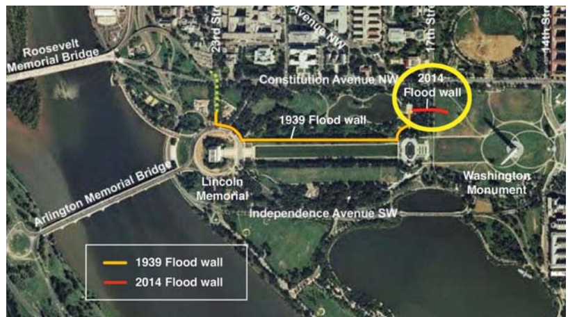
FEMA’s new floodplain map (above left) led to the decision to build the flood wall. Finished in 2014, the wall closes a gap in the flood control levee built in 1939 (orange line, map above right). The old plan to fill the gap with sandbags was deemed inadequate after Hurricane Katrina. MAPS, NATIONAL CAPITAL PLANNING COMMISSION
