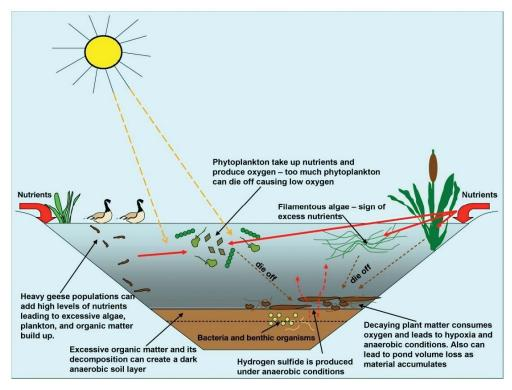
Biological and chemical processes resulting from nutrient inputs to a stormwater pond.
